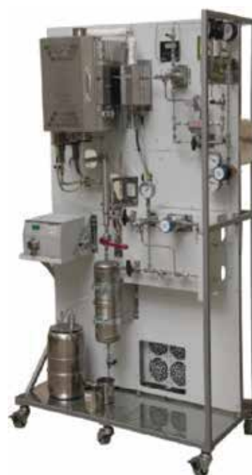
Autoclave with magnetic coupling volume 10 L, stainless steel with fluoroplastic coating, pressure 2MPa, temperature 200°C
